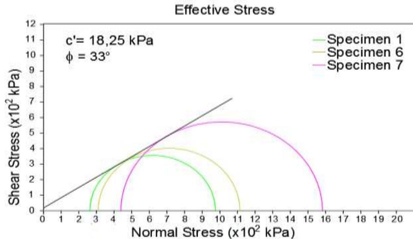
Figure 2: Mohr-Coulomb failure envelope for the 50mm diameter samples
