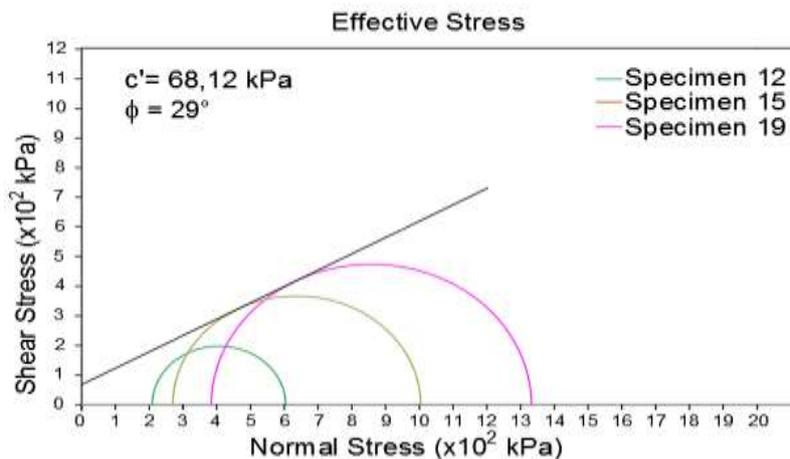
Figure 3: Mohr-Coulomb failure envelope for the 38mm diameter samples
