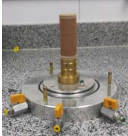
**Figure 1: Cylindrical specimen**
